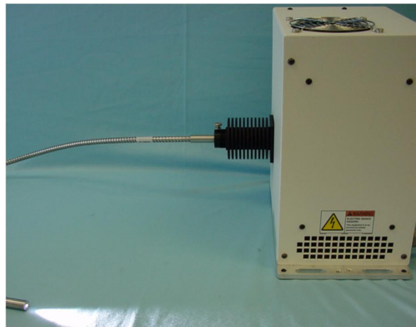
Abet Technologies Model LS 150 Light Source with a 20093 F/2 Fiber adapter and a fused silica fiber bundle
