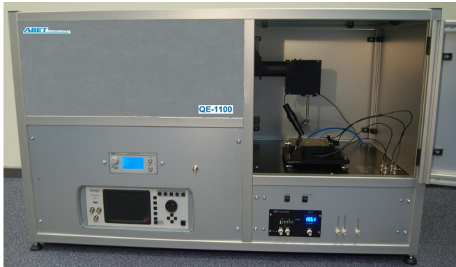
Abet Technologies Model QE-1100 Quantum Efficiency measurement tool, 350-1100 nm range
